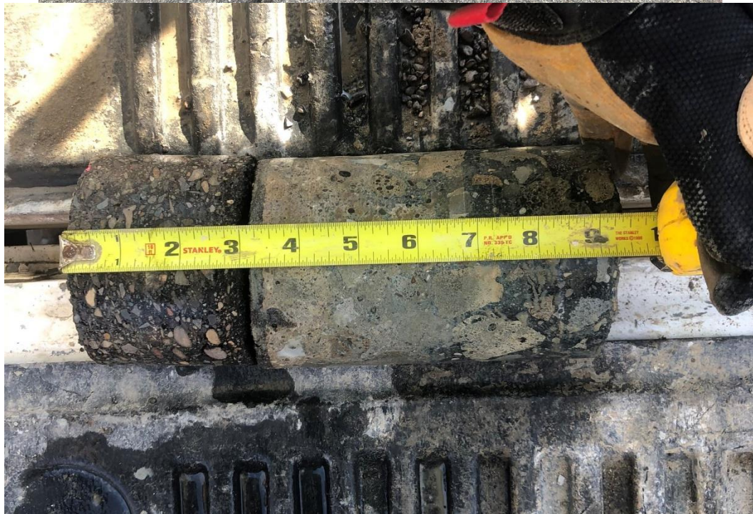
Photograph No. 5: Moderate to high severity transverse and longitudinal cracking with cold patching and full depth replacement patching near boring A-5. View to the west. Note the underlying Portland cement concrete contains slag aggregate.
