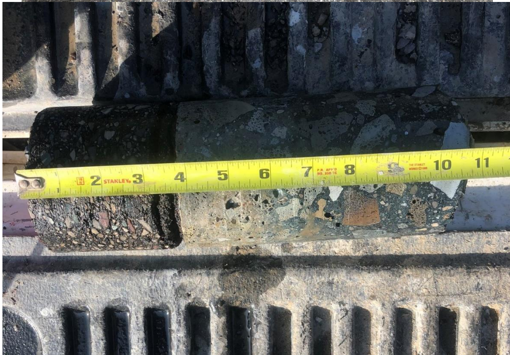
Photograph No. 6: Moderate severity transverse and longitudinal reflective cracking and edge cracking with cold patching and crack sealing near boring A-6. View to the west. Note the underlying Portland cement concrete contains slag aggregate.
