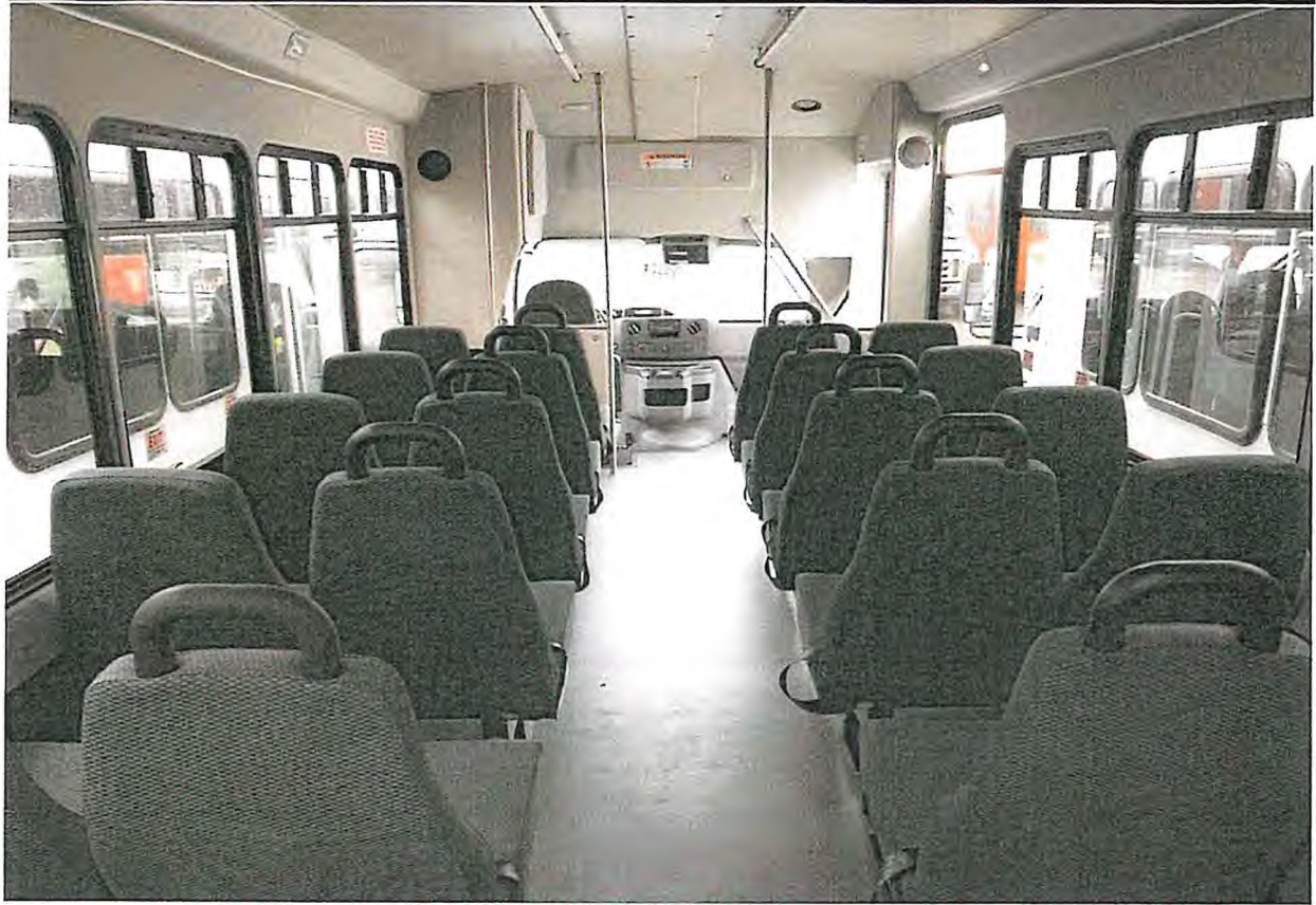
ACTUAL SEAT COVERING BELOW, JORDAN CLOTH ON SEAT BOTTOM AND FACE, BLACK VINYL TRIM AND BACKING.
