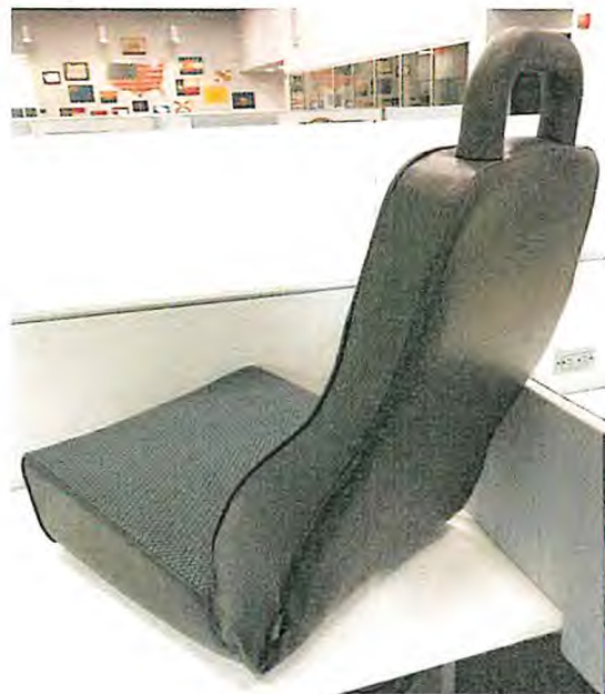
ACTUAL SEAT COVERING BELOW, JORDAN CLOTH ON SEAT BOTTOM AND FACE, BLACK VINYL TRIM AND BACKING.
