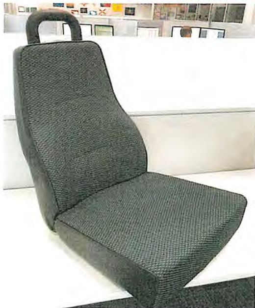
ACTUAL SEAT COVERING BELOW, JORDAN CLOTH ON SEAT BOTTOM AND FACE, BLACK VINYL TRIM AND BACKING.
